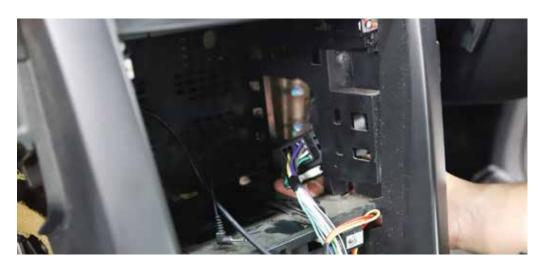
**Mounting the new facia**Run the temp sensor neatly to behind the radio and plug it into the facia
