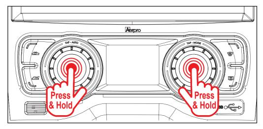
Press & hold both left & right rotary knobs at the same time.
