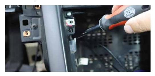
**Installing the temperature sensor**To install the temp sensor, you will need cable ties
