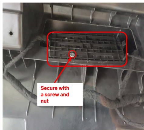
28 Secure the tailgate ECU bracket at that hole.
