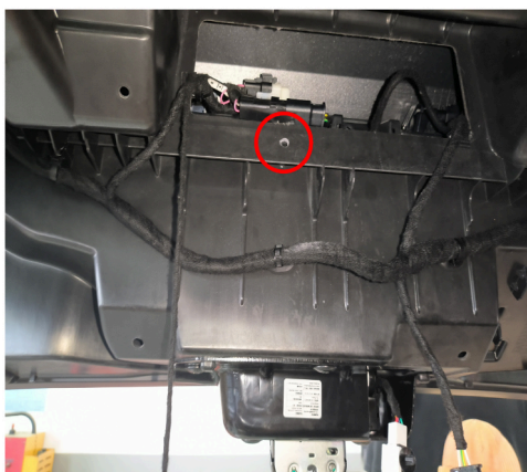
27 Drill a 6mm hole at the indicated position with the drill bit.
