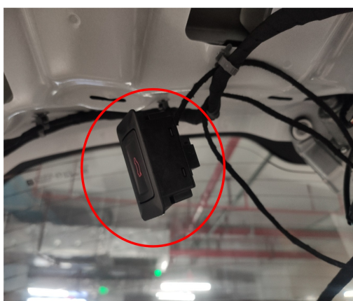
15 Connect the connector of the lock signal harness to the new tailgate switch.
