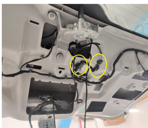
14 Connect the connectors of the lock signal harness to the factory tailgate switch.
