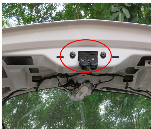
11 Remove the factory latch.
