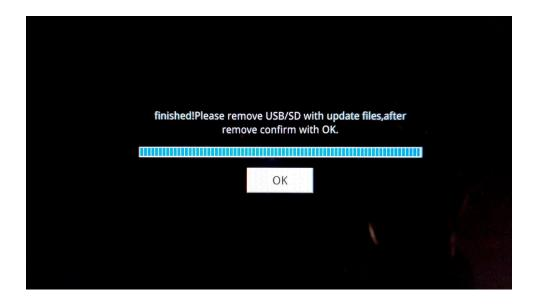
You will then be asked to **remove the USB BEFORE pressing the OK button** as the image above. Once the USB is taken out, you can continue by pressing the OK button on the screen. Pressing it once is sufficient, it will eventually restart. The update is now complete.
