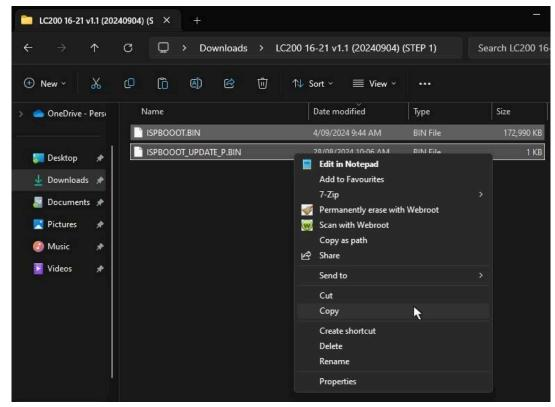
Once you have copied, navigate to your inserted USB drive and right click in the empty spot and click paste. There should be 2 files on the USB device. Safely remove the USB device and move back to your vehicle to install the first step firmware.
