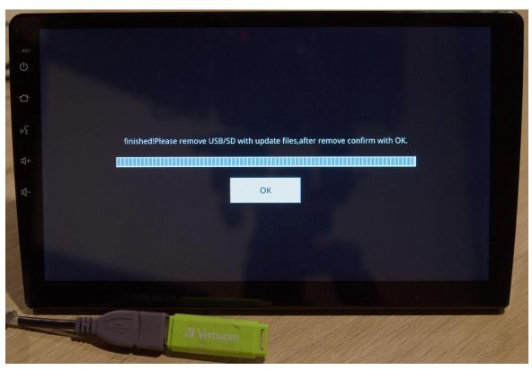
Once the head unit is finished restarting, it is recommended to turn off the car, wait 30 seconds then turn it back on. Then you can check the date number to make sure it has updated successfully and you may change the settings to your taste.
