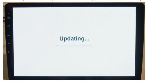
Once the headunit is finished updating, it will reboot and show the home screen/radio. **Disconnect** the USB device & Turn off the car, wait 30 seconds then turn it back on. Then you can check the date number to make sure it has updated successfully and you may change the settings to your taste.
