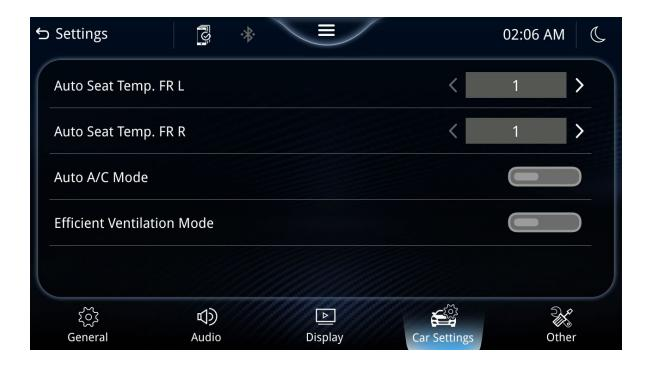
**Auto Seat Temp. FR L** - Adjusts sensitivity of the passengers seat when on Auto to engage sooner or later depending on setting. (Sahara variant only)
