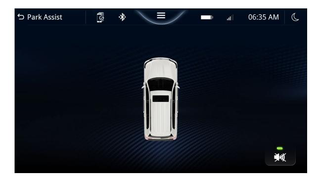
If the 'Display On-Screen Radar' setting is enabled, then this screen will appear whenever one of the front sensors detect an object under the following conditions.
