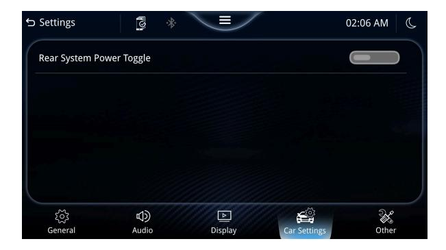
The Rear System Power Toggle allows you to remotely turn the rear entertainment systems on or off via the head unit. This is a toggle button and will simple toggle power regardless of current state.
