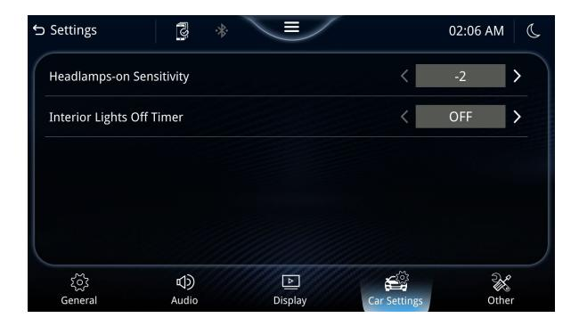
**Headlamps-on Sensitivity** - Adjust the sensitivity of headlamps to automatically turn on under sooner darker lighting conditions.
