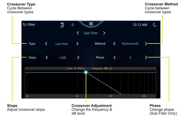
On this page you can adjust the crossover of the Subwoofer (if equipped), Front Speakers\* & Rear Speakers\*.
