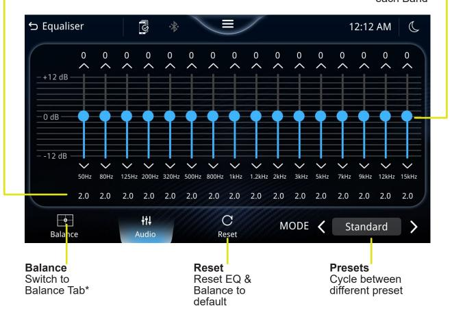
Selecting Equaliser from the Audio Menu Bar will bring up the 16 band graphic equaliser and presets. There are a 7 factory default presets with 3 custom presets to switch between. Frequency adjustments can be made by touching and sliding the sliders up/down. You can also adjust the Q-Factor by tapping the numbers underneath the band frequency. That will bring up a text box to change and apply the new Q-Factor Value.
