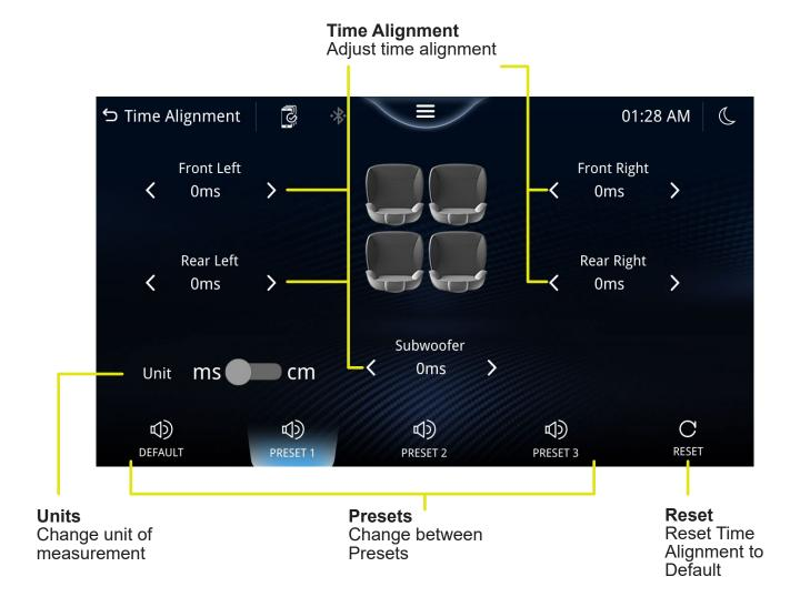
In order to begin making adjustments to time delay, you will have to switch to one of the presets. Once selected, you will now be able to adjust the time delay by using the arrows next to each speaker and subwoofer. If you would like to use cm's as a form of measurement, then using the Unit toggle on the left corner.
