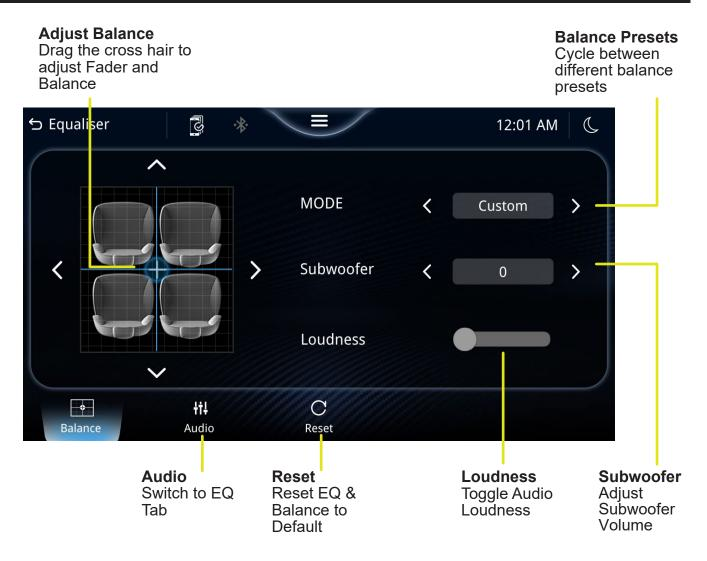
NOTE: if you are on any of the default presets and begin to make changes to the EQ then it will automatically switch over to the custom preset and overwrite any existing changes in the custom preset.
