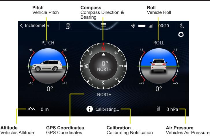
The inclinometer works by using the head units GPS and internal sensors to provide pitch, roll, bearing and GPS coordinates.
