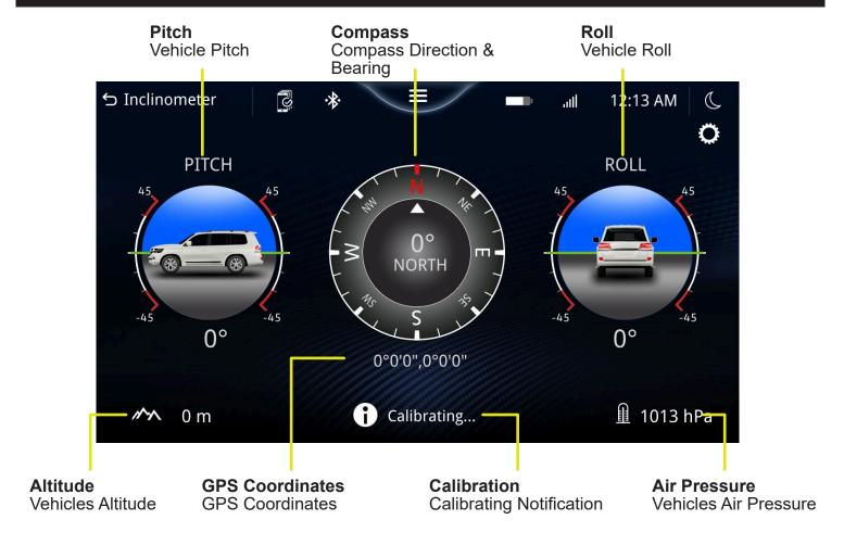
The inclinometer works by using the head units GPS and internal sensors to provide pitch, roll, bearing and GPS coordinates.
