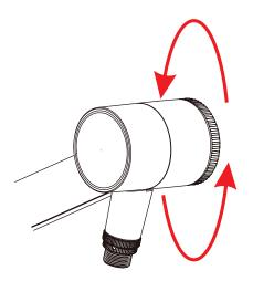
4. You can adjust the tension due to the weight of the microphone by tightening the adjustment screw near the base as pictured below. Tension is preset at about 50% and the load is about 0.8-1-0kg. If adjusted to the tightest state the maximum load is 1.5kg.
