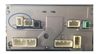
Connect the APVTY14C 4 pin connector to the factory head unit.
