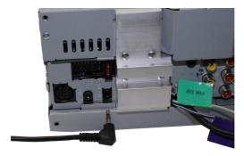
4. Connect the 14 way molex connector to the interface
