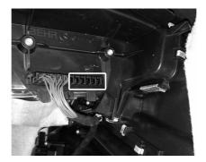
9. Connect the 8-Way connector to the MOST Interface
