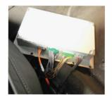
8. Disconnect the vehicle display and plug in the male green vehicle display connector. Take the disconnected display lead and plug this into the female green vehicle display connector
