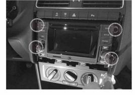
Remove the OEM head unit by unscrewing the four screws circled.
