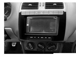
Mount the supplied facia plate on the dashboard. The image shows the final result.
