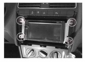
Connect all cables, insert the unit into the housing and fix it with the screws; verify the proper functioning of the system, including the touch buttons on the facia plate.
