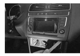
Carefully unclip the original panel. We reccomend using panel removal tools to avoid any damage.
