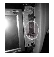
Before fitting the unit, cut and remove the two pivots on either side, as shown in the picture.
