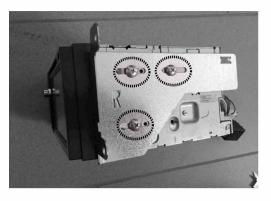
Take the left and right brackets and mount them on the unit using the screws supplied.
