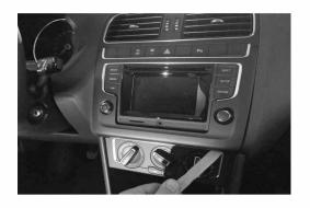
Carefully unclip the original panel. We recomend using panel removal tools to avoid any damage.
