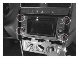
Remove the OEM head unit by unscrewing the four screws circled.
