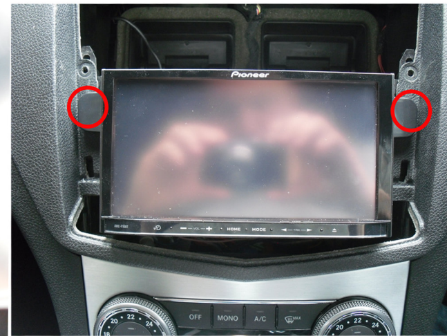
Ensure all wires are clear of the aperture. Slide the head unit back into the dash. Ensure that the guide knobs are lined up with the guide rails as shown.
