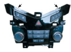
Cut out two edges from the OEM panel in order to clear space for Double DIN head unit (see arrows)
