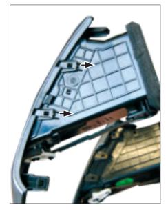
17. Remove the air vents of the original panel (left and right)
