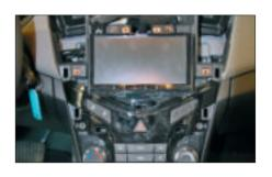
13. a: Mount the Double DIN head unit to the dash board and fix it with the original screws
