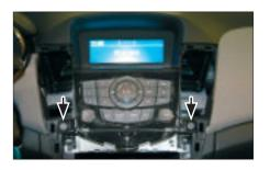
7. Remove screws of OEM radio (see arrows)
