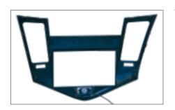
16. Clip speaker on new facia plate. Cable has to be fixed as shown on sample picture
