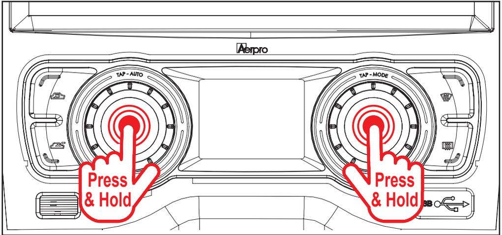
Press & hold both left & right rotary knobs at the same time.
