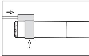
Align the attachment with the recessed groove on the camera head. Then clip the attachment together to firmly secure it to the camera head.
